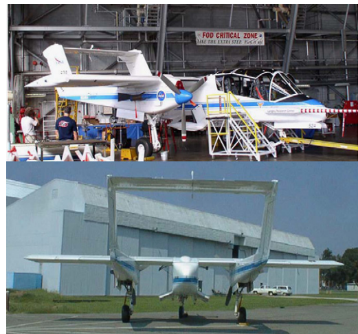
Fig. 9.1. The NASA LaRC OV-10 experimental aircraft with two cameras at the wing tips and one camera at the top of the left vertical tail.
