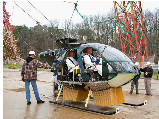
Fig. 7.30. MD-500 helicopter airframe being prepared for crash test with 4 crash dummies inside and 2 deployable energy absorbers beneath.
