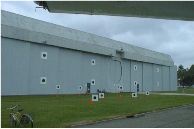
Fig. 9.3. Target field for camera calibration/orientation.
