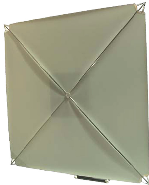
Fig. 10.7. Two-meter four quadrant Vellum solar sail test article.
