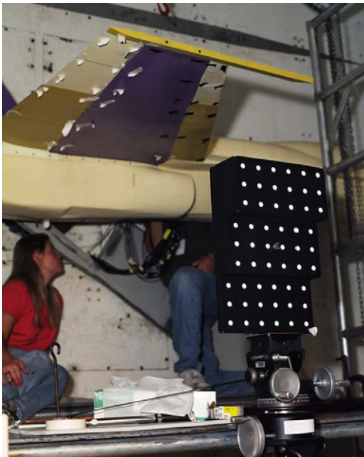
Fig. 4.13. Preparation of camera orientation using a step calibration target plate aligned with the tunnel coordinate system.
