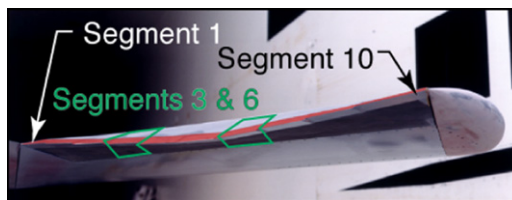
Fig. 7.1. Photograph of the “smart” trailing-edge control surface highlighting the segments monitored by VMD.
