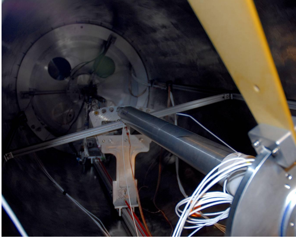
Figure 1. e^+e^- pair detection setup inside the HELIOS solenoid. The HELIOS silicon array is behind the target fan. In front of the target fan is the collimator tube that shields the SiLi detectors (not visible in this view) from alpha particles from the target.
