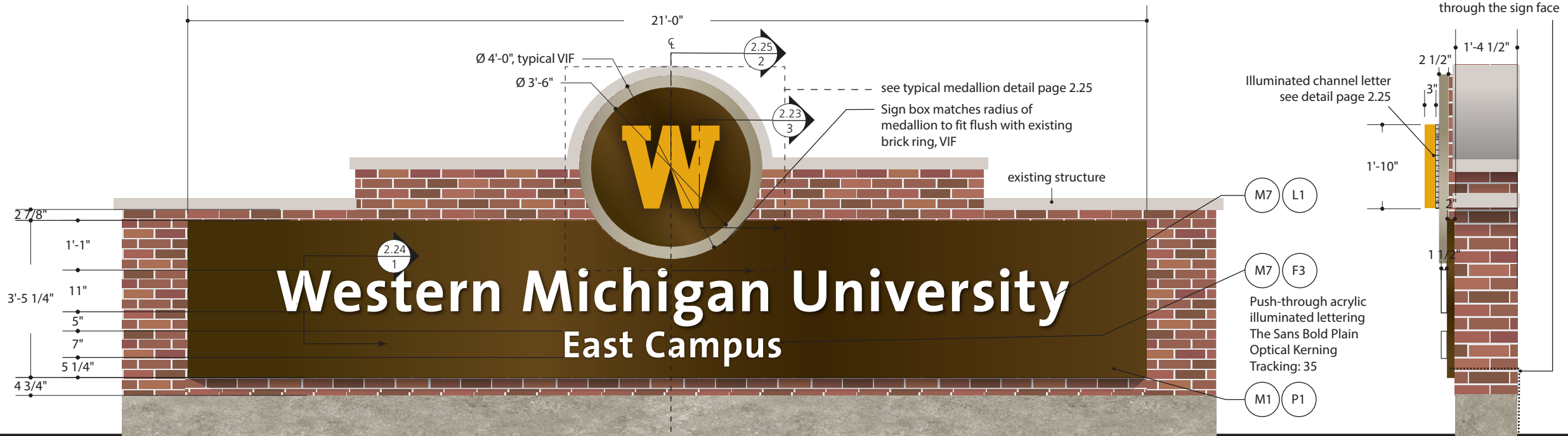
1 Elevation – Retrofit – GW05 - Oliver and Oakland Dr scale: 3/8" = 1'-0"
