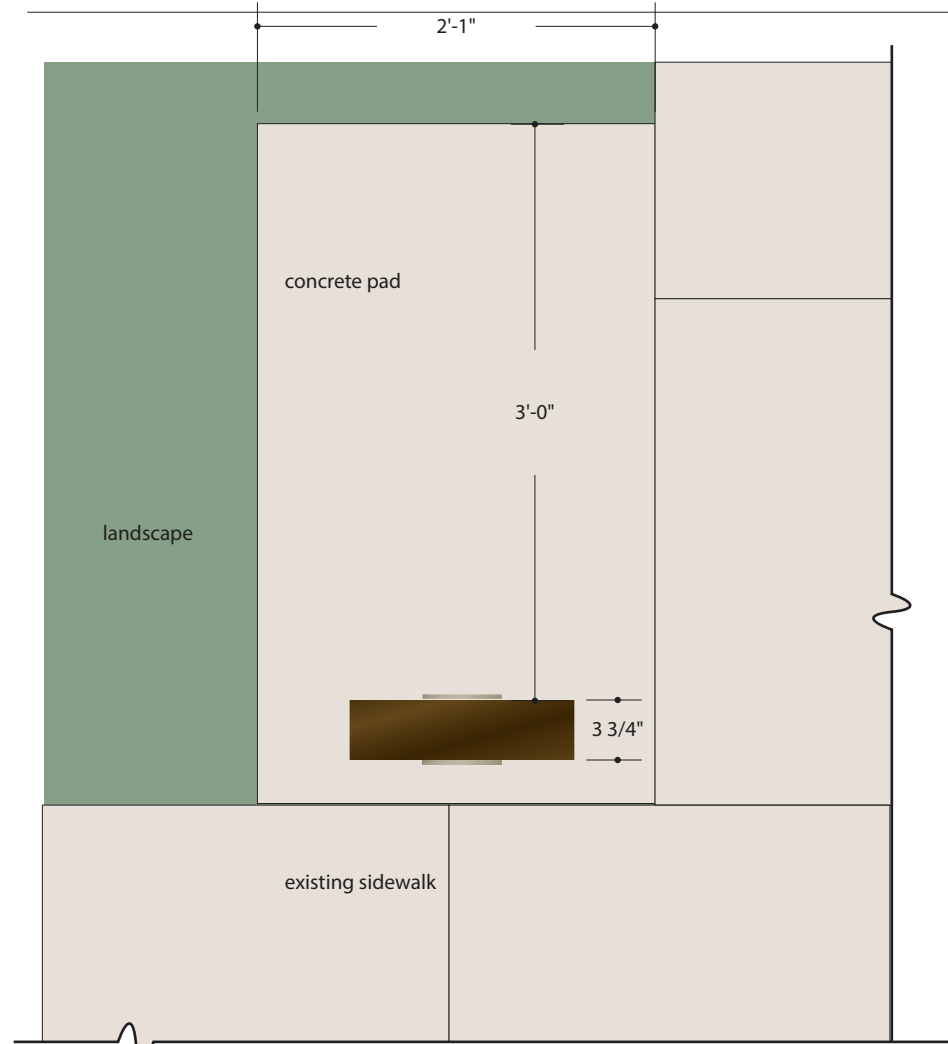
Plan view - Pedestrian directional pad - corner condition
