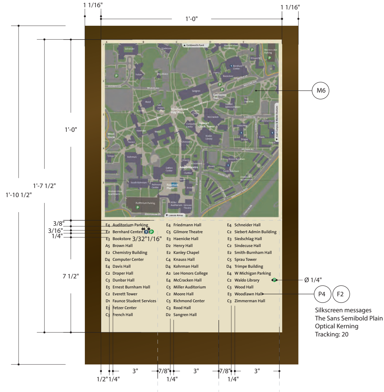
1 Layout – Map panel – ST 27 Ped Directional w/ map scale: 3"= 1'-0"
