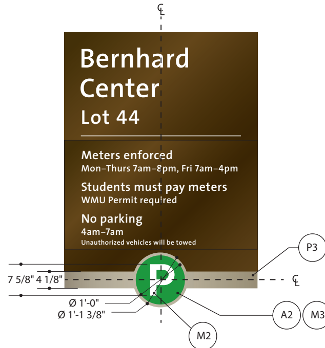
3 Typical Parking Band Layout - ST14 scale: 1/2"=1'-0"
