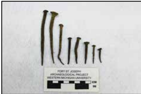
Figure 82. The most common nail type found at Fort St. Joseph are rose-head nails with pointed shanks.
