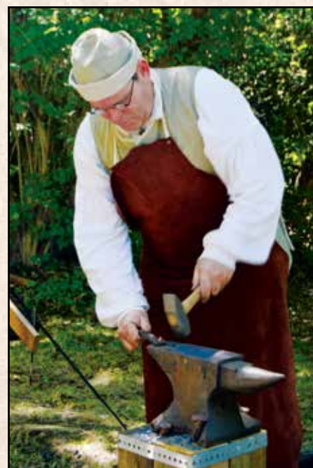
Figure 72. A reenactor at the 2016 Fort St. Joseph Archaeology Open House demonstrates how blacksmiths work iron to produce a variety of materials.
