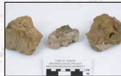
Figure 55. Many pieces of bousillage have been found during excavation at Fort St. Joseph. The piece on the left demonstrates how this material was packed around rounded posts for insulation. The center and right pieces depict the presence of white wash used to protect the walls from the elements.
