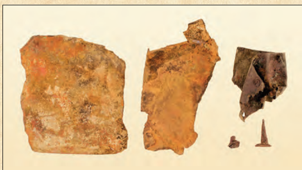
Figure 24 · Copper scrap, patches, and rivets served to prolong the use of kettles.
