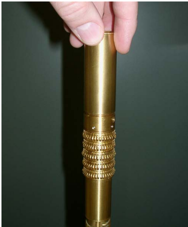
Figure 4-1. The radiation shield unscrews from the condenser tube.
