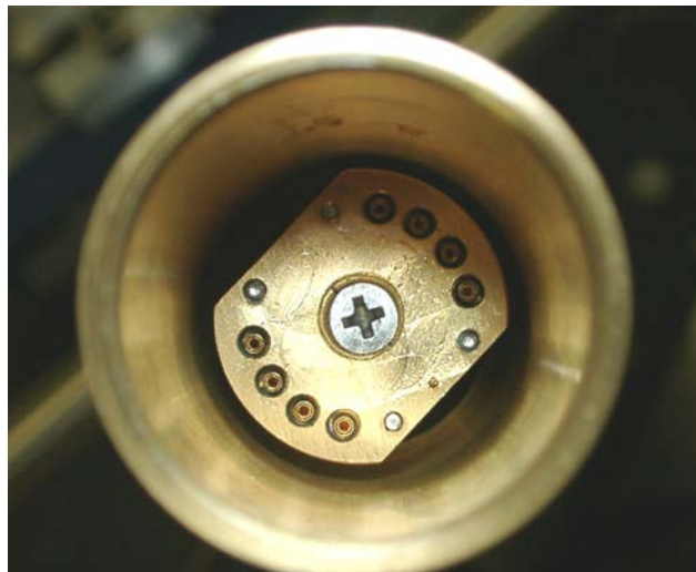
Figure 4-4. Ensure there are no touches between the sample stage and radiation shield.
