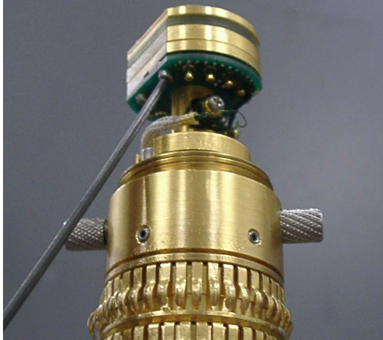
Figure 4-3. Tighten hex screws on sample stage.
