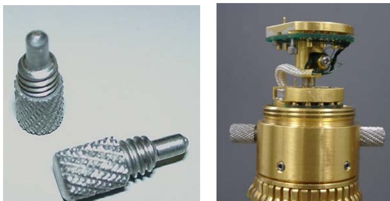
Figure 2-15. Sample mounting pins used to secure the mixing chamber.
