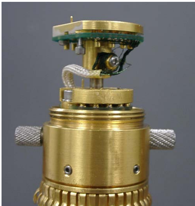
Figure 4-2. Install sample mounting pins prior to mounting or dismounting samples.
