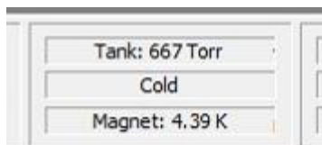
Figure 1-2. Cryostat monitor status panel showing “Cold” cryostat.
