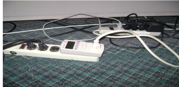
2. Use of two power strips required due to design of power meters.
