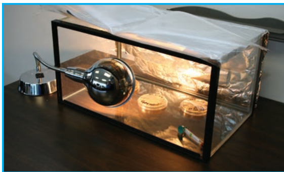
Image 3: Incubator made from a 10-gallon aquarium with open plastic cover.
