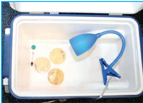
Image 1: Incubator made from a hard-side cooler.
